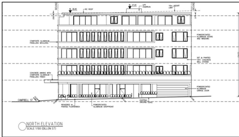
Figure 24: Extract from architectural drawings depicting the extent of non-compliance relative to the 16m statutory height limit along the northern (Dillon Street) elevation.
