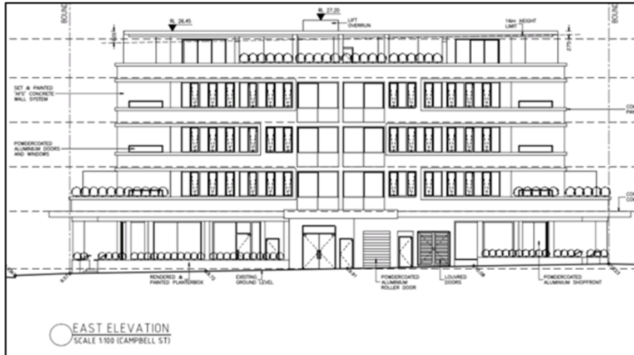
Figure 22: Extract from architectural drawings depicting the extent of non-compliance relative to the 16m statutory height limit along the eastern (Campbell Street) elevation.
