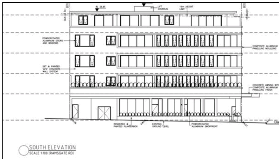
Figure 23: Extract from architectural drawings depicting the extent of non-compliance relative to the 16m statutory height limit along the southern (Ramsgate Road) elevation.
