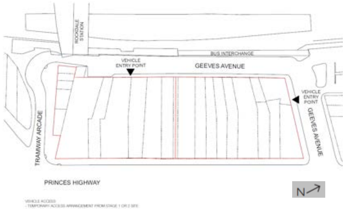
Figure 7.5.25: Temporary access solution for Stages 1 and 2
