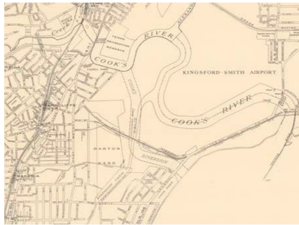
Figure 2.2 - The map shows the original Cooks River alignment and proposed realignment of Cooks River.
