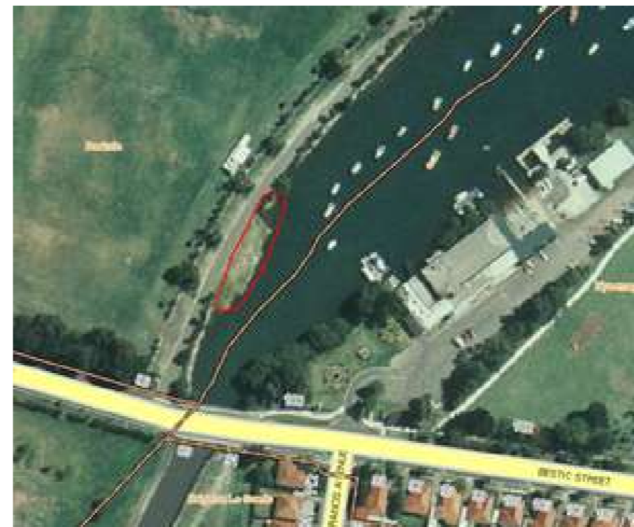
Figure 2.8 - Year 2000 aerial photograph shows extension of bank of Muddy Creek. This has effectively added reclaimed land to the banks of Barton Park
