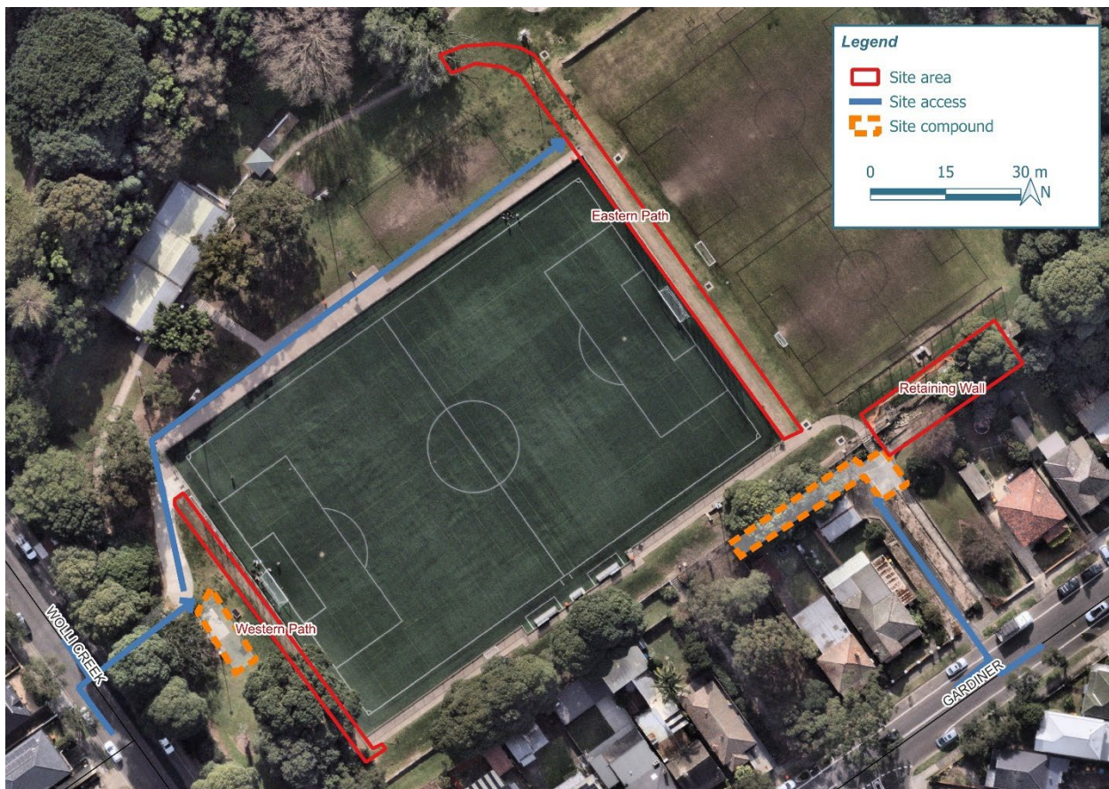
Figure 1-9: Proposed site access and area(s) suitable for site compound facilities (e.g., material storage, excavator laydown) for the proposed concrete pathways
