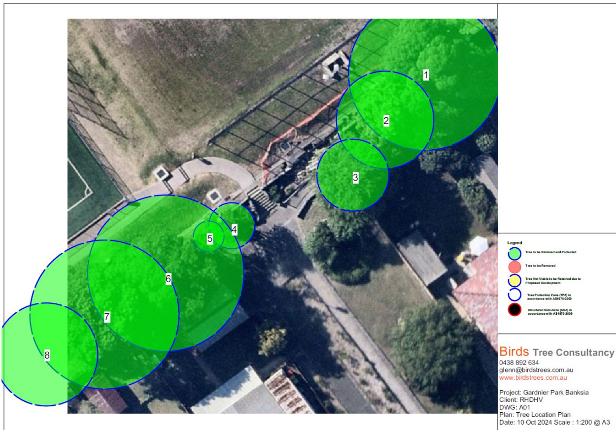
Figure 4-11: Proposed retaining wall Tree Protection Zones (TPZs)
