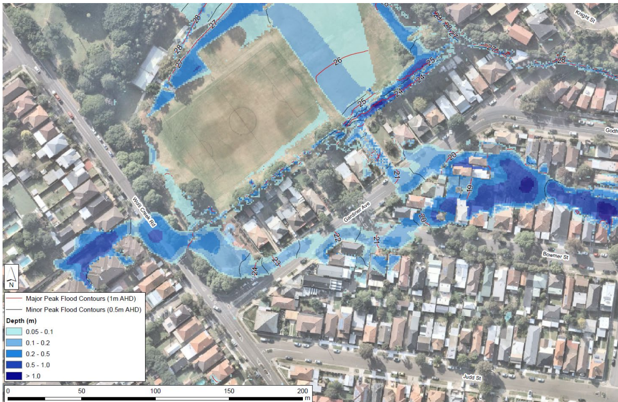
Figure 4-5: Post-development flood mapping for a 20% AEP event (WMA, 2024)
