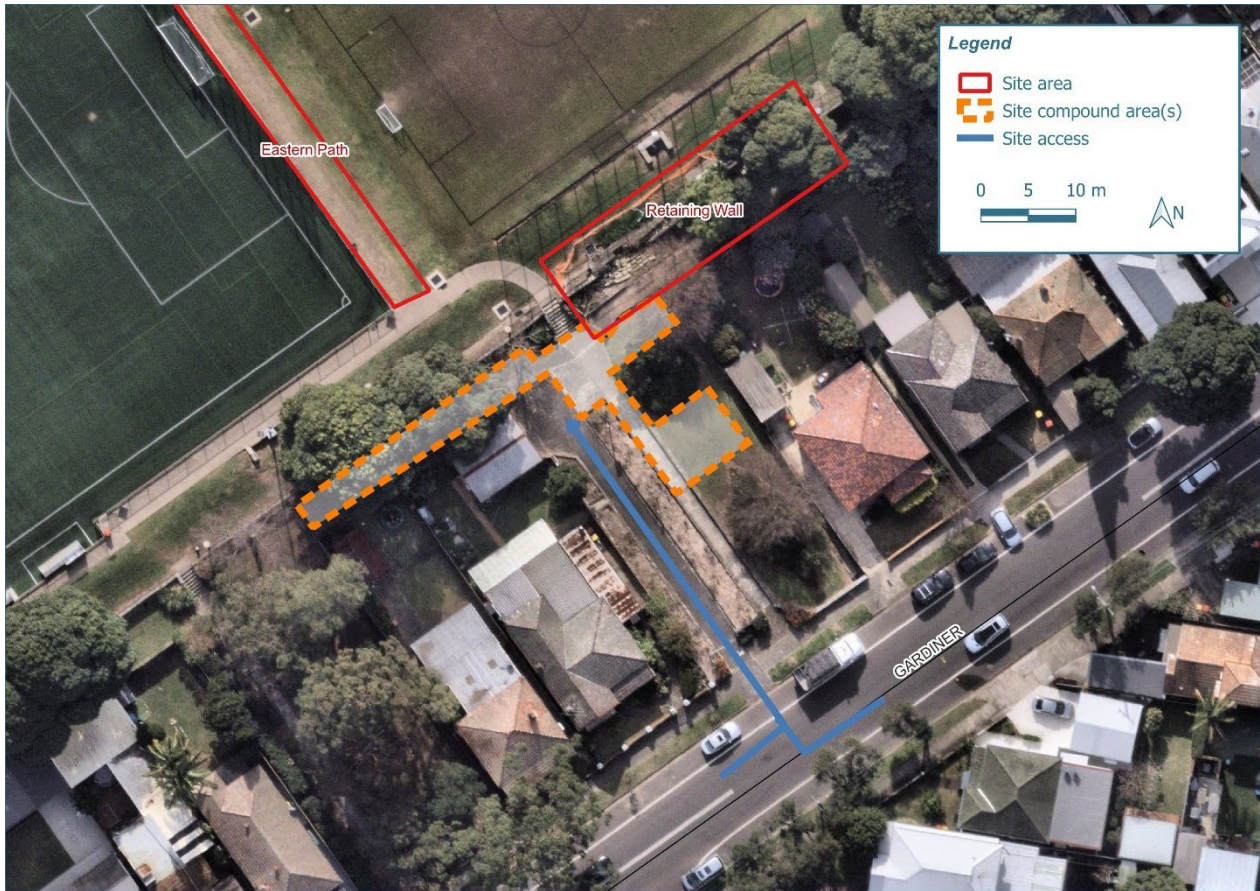
Figure 1-6: Proposed site access and area(s) suitable for site compound facilities (e.g., material storage, excavator laydown) for the proposed retaining wall remediation
